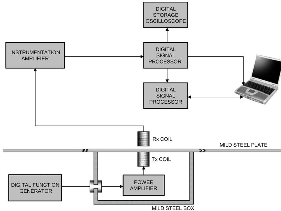
Fig. 1. Instrumentation configuration.
