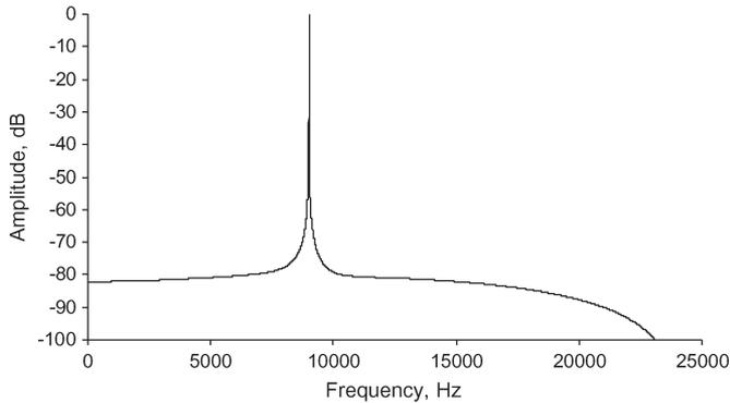
Fig. 3. Frequency response of the super narrow-band filter at 9 kHz. Note the decibel scale of the amplitude axis.
