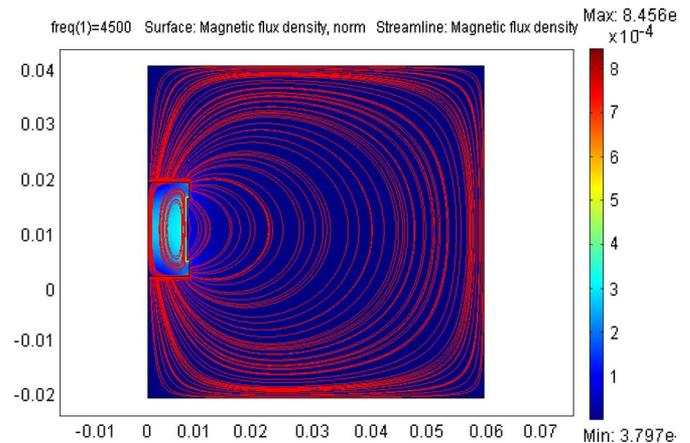
Fig. 2. Finite-element image of the transmitter coil produced by the modeling package *Femlab*, with which the magnetic field density at the top surface of the coil was estimated.
