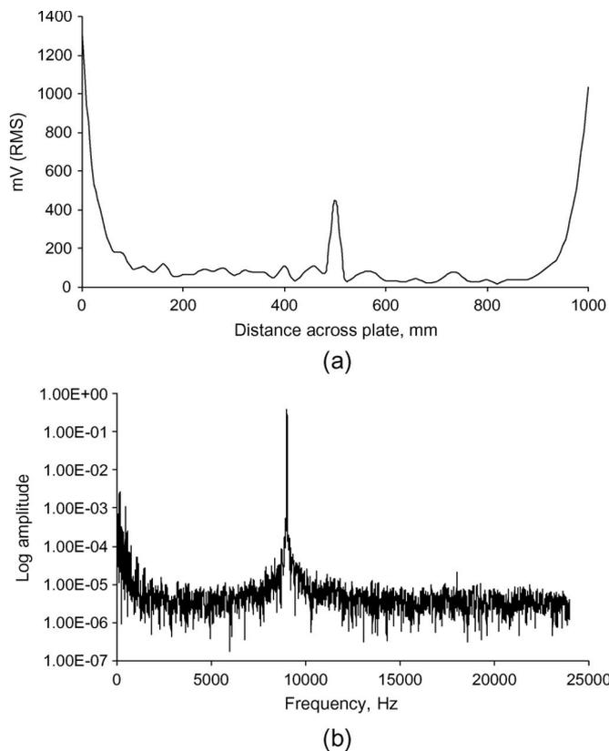
Fig. 5. (a) Line scan result at 9 kHz and a liftoff of 3 mm. (b) Fourier spectrum of the processed signal with the receiver coil located above the transmitter.
